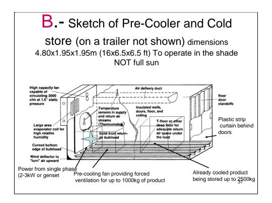
Note: Although the diagram shows the container with a T bar floor, this is not necessary and a standard non slip floor used in a cold truck would be adequate.
