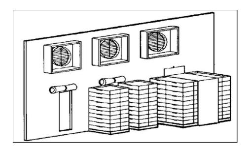
Sketch of a cooling wall for forced cooling of product, the air is sucked through the cartons and then blown back into the room through the fans. For this case two openings rather than three are suggested.
